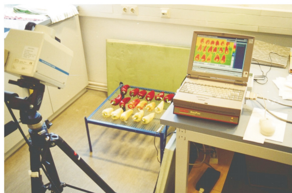
Fig. 2 Picture of the surface thermal imaging system (Varioscan 2011)
